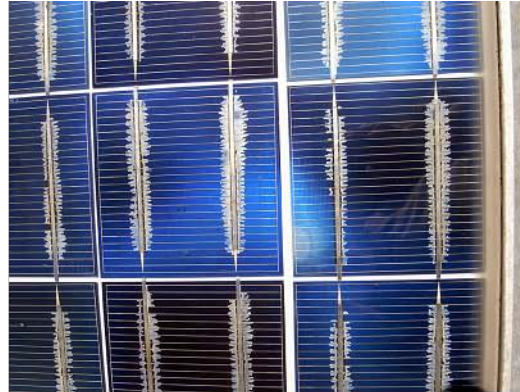
Delamination of encapsulant
