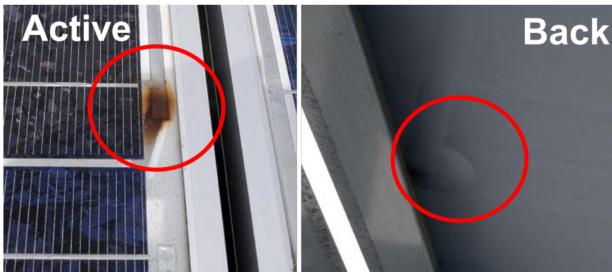
Overheat of connection area of bus ribbons
