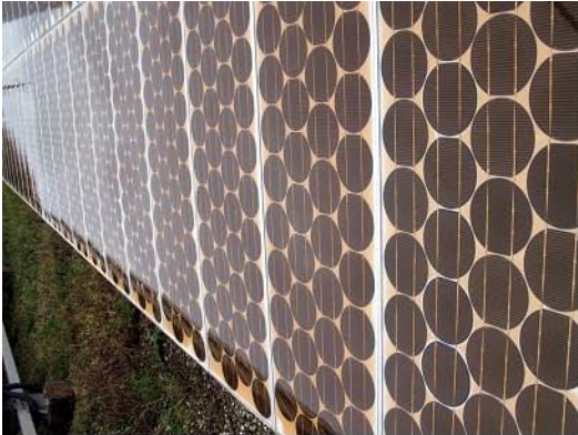
Yellowing of encapsulant
