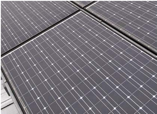
Subtle yellowing of encapsulant
