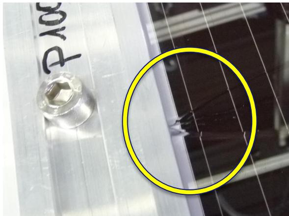
Cracks starting from edge of clamps
