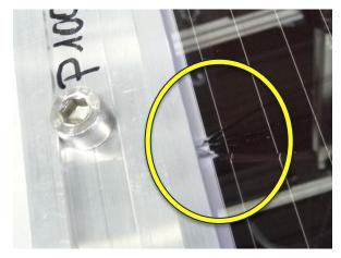
Cracks starting from edge of clamps
