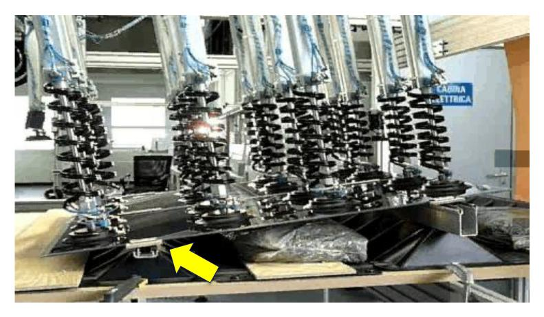
Flat roof system for glass – glass modules with fast clamping system
