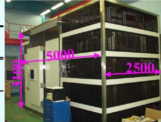
Acceleration Test: UV-Thermal Combined Stress
