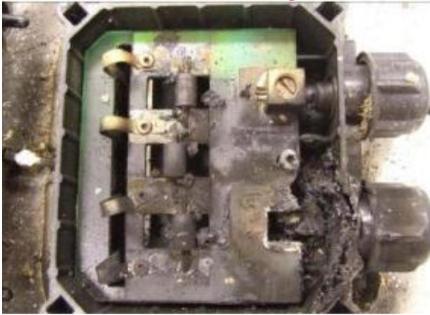
Solder Joint Degradation
