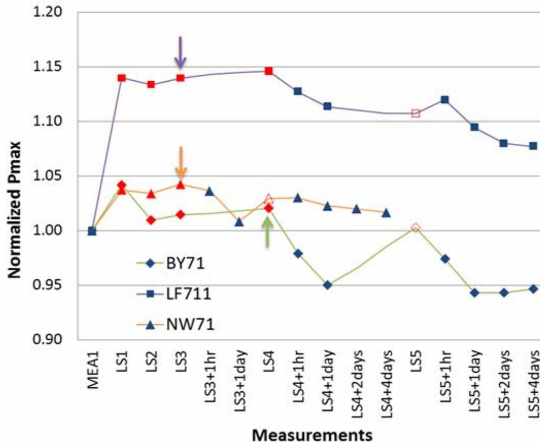
Modules measured within 30 minutes of leaving the light-soaking chamber
